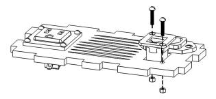
Mount the ethernet receptacle to acrylic face in the final mounting hole. Mount the receptacle by running bolts through the external face and securing these to nuts on the inside face of the acrylic.
