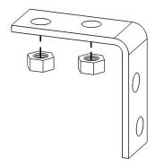
Prepare the L-bracket by gluing nuts to two of the holes. These nuts will be used to secure the top of the enclosure once the module is fully assembled.
