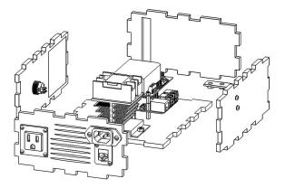
Attach the acrylic faces as shown. Note the orientation of each face. As shown in the image, the lasercut mounting slot for the card slot assembly should be located on the side of the enclosure with the button. Attach these faces by pressure fitting them, using glue, or using an acrylic solvent.
