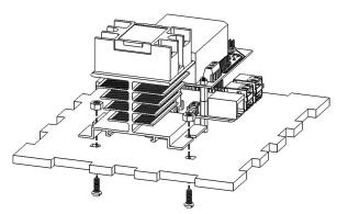
Next mount the SSR and heat sink assembly to the acrylic. This assembly should be mounted by running bolts up through the bottom of the acrylic and screwing them into nuts placed on the mounting slots in the heat sink. Note that the SSR should be oriented with the terminals labeled 1 and 2 to the left in the image shown and the terminals labeled 3 and 4 to the right in the image shown.
