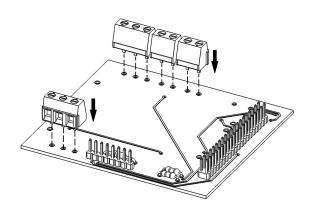
Mount the four terminal blocks to the PCB. Each block should be mounted such that wires can be inserted from the outside edge. If these terminal blocks are inverted, there will not be adequate room to insert wires. Solder the exposed through-hole pins on the bottom side of the board.
