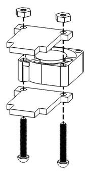
Attach the cooling fan to the 1/8" acrylic fan mounts as shown. Note that in the shown orientation, airflow will be directed toward the side of the mount on which the nuts are attached.
