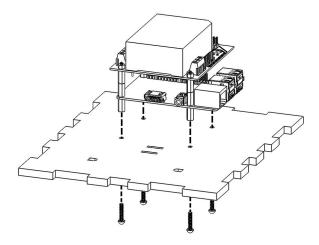
Begin assembling the final enclosure by mounting the previous assemblies to the enclosure's bottom lasercut from ¼" acrylic. First mount the Raspberry Pi and PCB assembly. Screw bolts through the mounting holes in the acrylic and up into the threaded bottoms of the standoffs.
