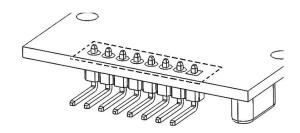
Reversing the board, solder the pins to the exposed pads on the underside. Set the RFID reader module aside for now.
