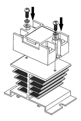
Mount the solid state relay (SSR) to the heat sink using the bolts and washers provided. Note that the smaller of the washers will be placed on the bolt first and the larger of the washers will contact the SSR directly. It is important in this step to **use thermal paste** between the SSR and heat sink. Place a small amount of thermal paste on the underside of the SSR before mounting it.
