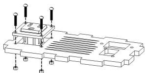
Continue assembling the module by mounting the outlet assembly to the rear acrylic face lasercut from ¼" acrylic. Begin by mounting the outlet assembly by running bolts through the external face and securing these to nuts on the inside face of the acrylic.
