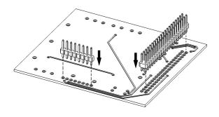
Mount the 1x8 and 2x20 header pin arrays to the PCB. Solder the exposed through-hole pins on the underside of the board.
