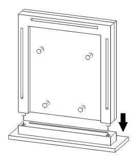
Attach the slot you have just created to the top portion of the card slot assembly. Again ensure that these pieces properly align as inverting either piece will impede the card's path when inserted. Once you have ensured that the pieces fit securely and a card can easily be inserted, attach the pieces using glue.
