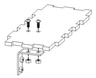
Mount the prepared L-bracket to the lasercut acrylic side of the enclosure. Mount The L-bracket by running bolts through the external face and securing these to nuts on the inside face of the L-bracket.
