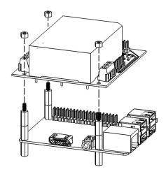
The PCB can now be mounted on top of the Raspberry Pi by aligning the mounting holes in the PCB with the standoffs. Note again that only three of the four mounting holes will be used.
