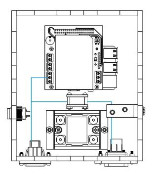
The blue line in the shown image traces the path of the white 14 or 16 AWG neutral wire. Note that the wire passes underneath the cooling fan assembly in the space between the fan mounts. Note also that there is a direct electrical connection between the inlet and outlet.
