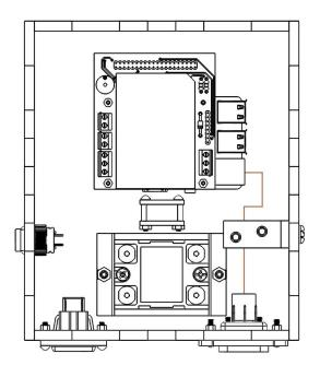
If ethernet will not be available in the target resource location, skip this step and continue. If ethernet will be available in the target resource location, connect an ethernet patch cable from the ethernet port of the Raspberry Pi to the ethernet receptacle mounted on the rear acrylic face of the module enclosure.
