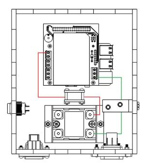
The paths shown in the accompanying diagram are for the signal leads of the SSR. The green line represents the ground wire that should be attached to terminal 4 on the SSR. The red line represents the positive signal wire that should be attached to terminal 3 on the SSR.
