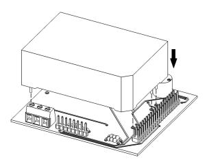
Mount the AC to DC converter to the PCB. The converter will only fit in one orientation due to the asymmetrical pin locations. Solder the exposed through-hole pins on the bottom side of the board.
