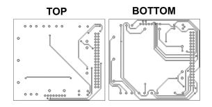
You will now begin assembling the printed circuit board (PCB). Ensure the board is in the proper orientation before beginning to mount components. Components will be placed on the top of the board but the through-hole pins will be soldered to the exposed pads on the PCBs bottom side.
