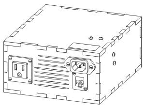
The module should now appear as shown. Place the adhesive rubber feet on the face that will serve as the bottom of the module. The module is now ready to be implemented. To implement, attach ethernet to the exposed ethernet port on the box (if using ethernet and not WiFi). Power can then be applied to the inlet using a 14 AWG power cord.
