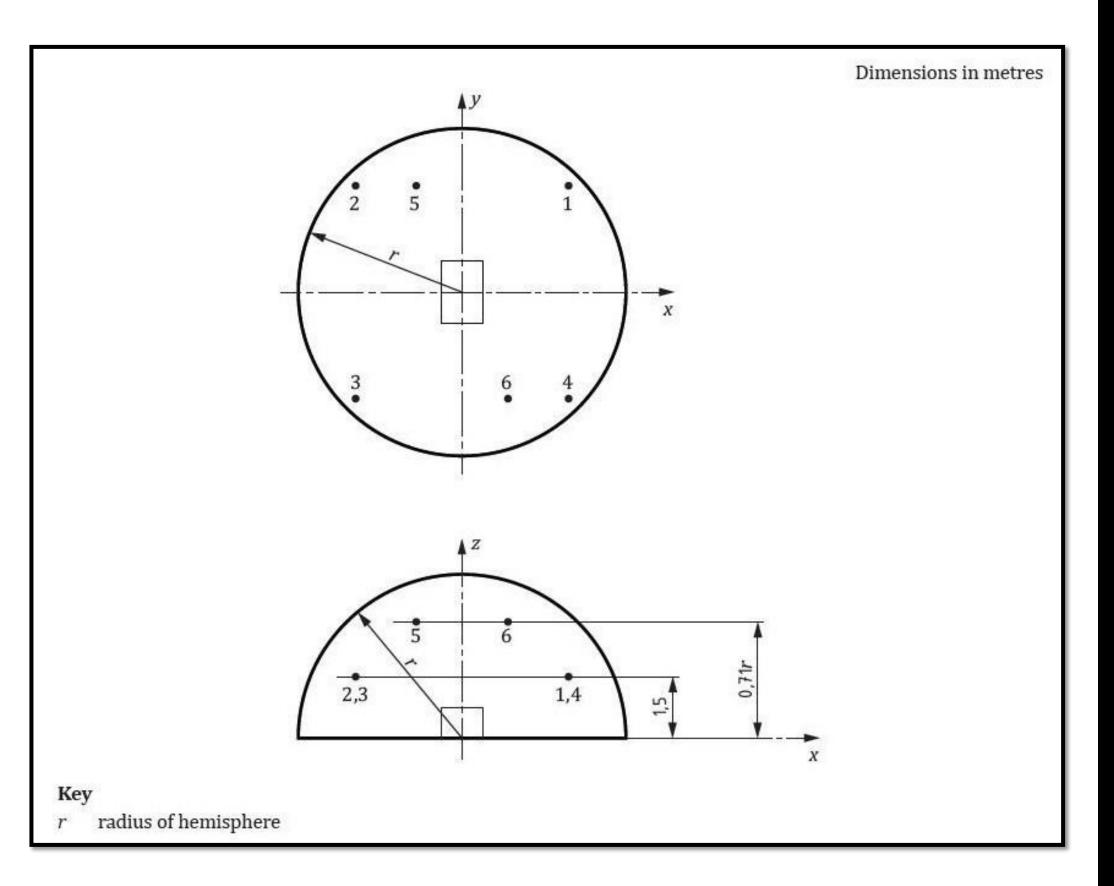
Figure 3. Sound level meter positions on the hemisphere (see Table 1).
