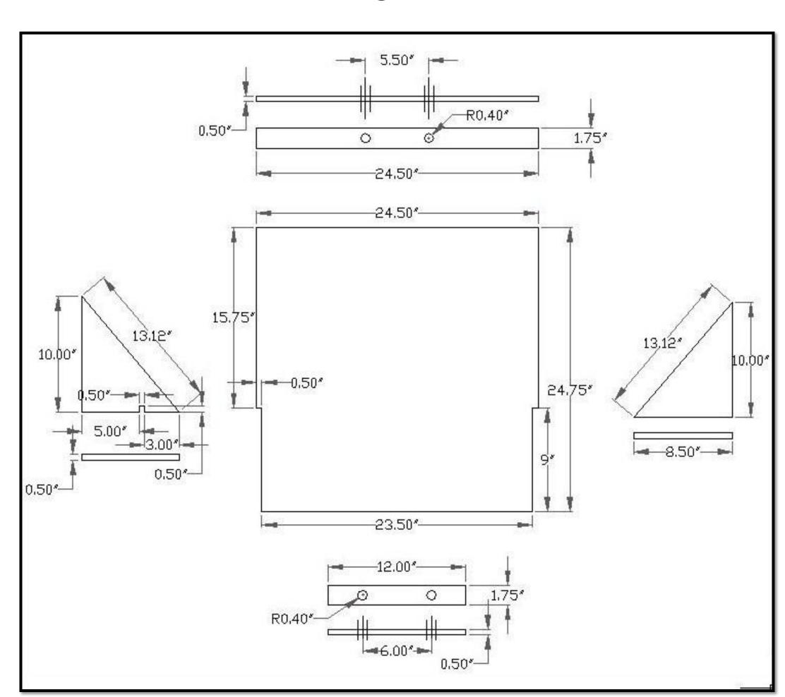
Figure 2. Technical Drawing of suggested shield design.
